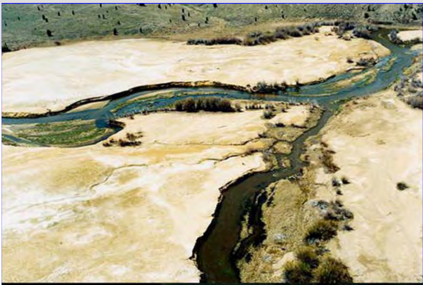
Silver Bow Creek at Ramsay Flats before remediation and restoration started. Clear evidence of tailings contamination is visible throughout the riparian habitat.
